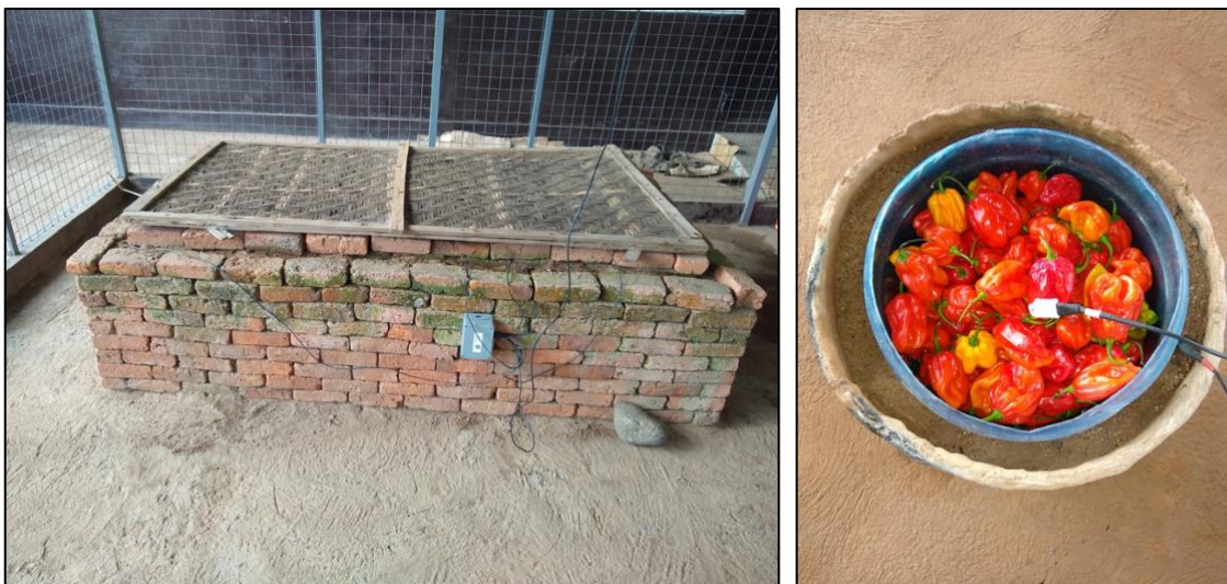
A brick Zero Energy Cooling Chamber (left) and a clay pot cooler (right) in Rubona, Rwanda.
