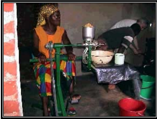
VitaGoat cycle grinder at work grinding soybeans for soymilk, Mozambique.
